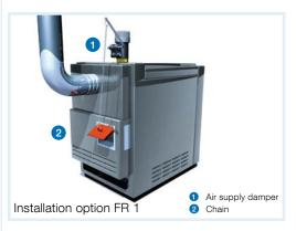
The FR 1 combustion controller controls the combustion air supply. The temperature in the heat generator is detected by an integrated thermostat. The thermostat is connected to the air supply damper by means of a lever and a chain. The air supply is controlled by means of opening or closing the air supply damper, depending on the boiler flow temperature.
